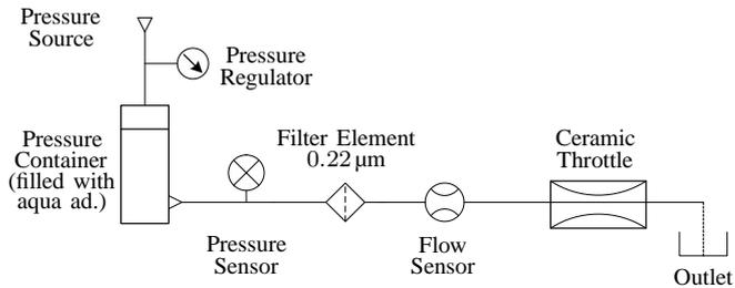
Fig. 4. Blockdiagram of measurement set-up
