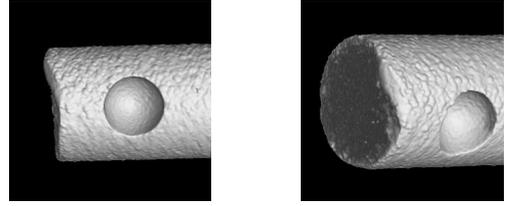
Fig. 3. Micro-CT of  $ZrO_2$ -cylinder front side in different views
