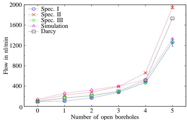
Fig. 5. Flow results of experiments, simulation and Darcy equation
