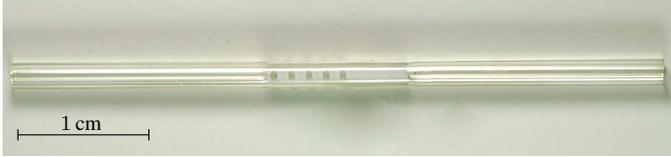
Fig. 1. Sample of manufactured  $ZrO_2$ -throttle
